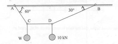
3. Determine tension in the cables AB, BC & CD.
