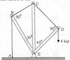
Determine support reactions at A & B and all other internal pins. Identify two-force members and determine the forces in those members. Assume all the members of the framework are weightless.
