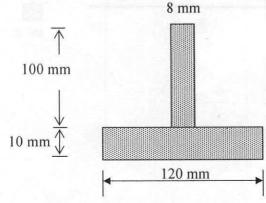
12. Calculate the moment of inertia of the following section about the X axis and Y axis.
