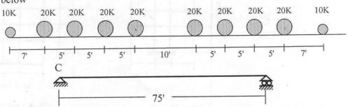
9. Calculate the maximum live load shear at the quarter point from the left support of a simply supported beam of span 100 ft due to the axle loads of a heavy freight locomotive shown below.
