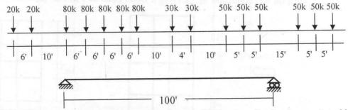
10. Calculate the maximum bending moment at the one-third point of a simply supported beam of span 70 ft due to the wheel loads shown in the figure below.
