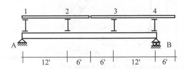
7. Draw the shear force and bending moment diagrams for the following structure.
