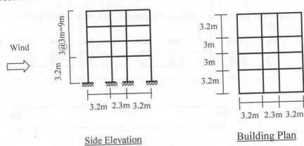
Calculate the seismic load at each story of a six-storied hospital building (shown below) located in Dhaka (Zone 2). Assume the structure to be an Ordinary Moment Resisting Frame (OMRF) built on soil condition S2, carrying a Dead Load of 9 kN/m<sup>2</sup> (Including partition load).
