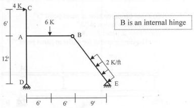
3. For the beam shown below, draw Influence lines for (i) Reaction at B, (ii) Shear at C, (iii) Shear just right of B and (iv) Vertical reaction at E (v) Moment at C.
