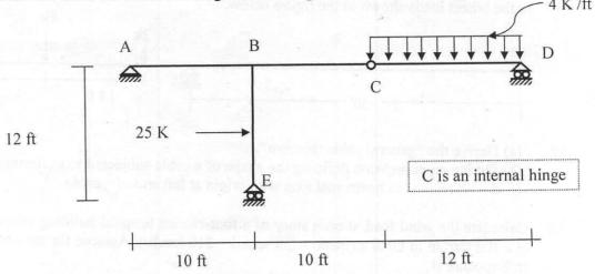
8. Calculate the maximum reaction at support C of a deck girder due to the loads as shown in the figure below
