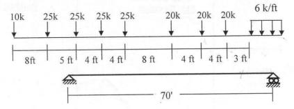
11. Calculate the absolute maximum bending moment of a simply supported beam of span 50 ft due to the wheel loads shown in the figure below. 8k
