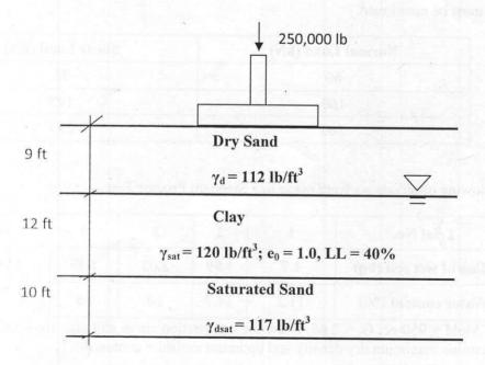
Given that: Cc = 0.009(LL-10); Stress increase at the top of the clay layer,  $\Delta\sigma_t = 0.055 *\sigma_{applied}$ ; Stress increase at the middle of the clay layer,  $\Delta\sigma_m = 0.028 *\sigma_{applied}$ ; Stress increase at the bottom of the clay layer,  $\Delta\sigma_b = 0.02 *\sigma_{applied}$ ; Average stress increase,  $\Delta\sigma = (2 \Delta\sigma_t + 4 \Delta\sigma_m + 3 \Delta\sigma_b)/9$
