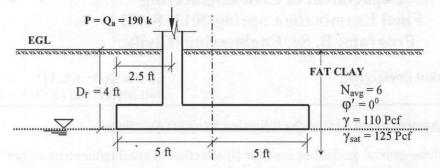
4. (a) Design the size of a rectangular combined footing for the conditions shown below  $(q_a = 2.0 \text{ tsf})$ .
