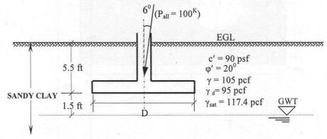
(b) Allowable load (FS=2.5) of an eccentrically loaded rectangular footing (Breadth as shown below) using Meyerhof's effective area method is 190 k. Determine the length of the footing.
